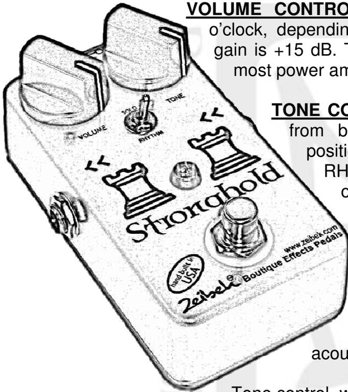
**VOLUME CONTROL:** Unity gain (0 dB) occurs at 9-10 o'clock, depending on the input signal. Maximum output gain is +15 dB. This is more than enough power to drive most power amps.
